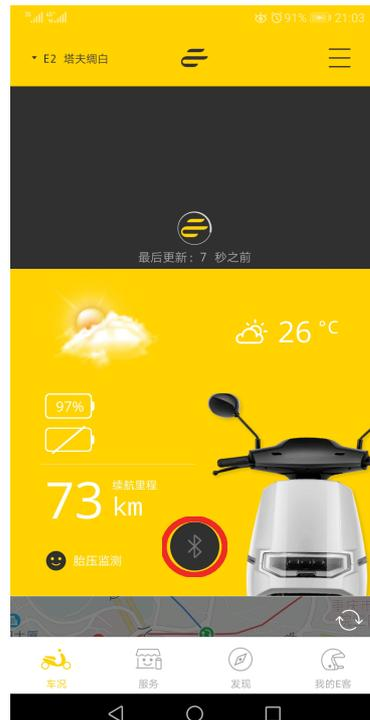
When the new scooter leaves the factory, MCU is the latest version , but in the process of warehousing, transportation, etc., the MCU may be updated. So when you receive the new scooter, please enter into the “Central Control Version” interface for query and update. If there is software update, there will be a red dot prompt.
