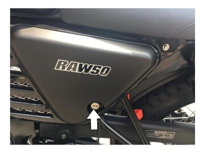
Above indicates the lock is the battery box protection cover, to take out the battery, please open the lock with a key switch.
