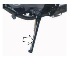
To use the main, depress it by foot and lift the rear of the motorcycle until the rear wheel is lift. To use the side, depress the end of it until it rotates to the end and stops.
