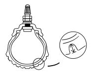
Operating the motorcycle with excessively worn tires will decrease riding stability and can lead to loss of control. It is recommended that a tire be replaced when the remaining depth of tire tread becomes 1.6mm or less.
