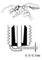
type of usage. If the standard spark plug is very black, you'd better use a high-pressure hot type of spark plug. A normal operating spark plug should be light brown or tan in color. If the color is white or seem flashing, it is used in overheat condition and change it with a cold type one.
